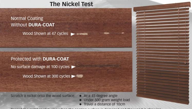
Record the number of cycles when the coating surface is damaged and the wood is showing.
